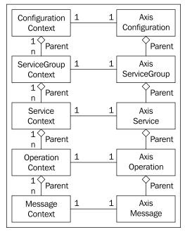
From the above figure, we can observe that the top-most component of the hierarchy is **ConfigurationContext**. The only difference in ConfigurationContext when compared to the other contexts is that it is the only context that exists in the system before a message is received. ConfigurationContext has a reference to an AxisConfiguration, and to create ConfigurationContext, it is required to have an AxisConfiguration available.
