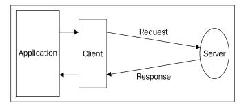
In case of asynchronous invocation, the user application (e.g. GUI) does not block, so the user can continue working. The Axis2 way of utilizing a service in asynchronous invocation is shown in the following figure:
