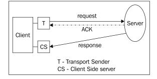
In order to invoke a service in the above manner, we need to have WS-Addressing support. We also need to engage the addressing module on both the client side and the server side. In Scenario 2, we only had an application-level asynchronous support, but here we have transport-level asynchronous support as well.
