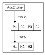
A phase is designed to support different phase rules. These rules include phaseFirst as well as phaseLast. In a phase, there are reserved slots to hold both phaseFirst handlers and phaseLast handlers. The rest of the handlers are in a different list. A phase can, therefore, be graphically represented as follows:
