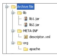
As mentioned earlier, the descriptor.xml file would be the services.xml file for a service. So in the service archive file, we can find a file named services.xml inside the META-INF directory. On the other hand, the module archive file will have a file named module.xml inside the META-INF directory.
