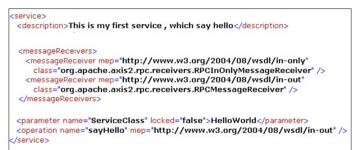
According to services.xml, the RPCMessageReceiver is the message receiver for all the in-out operations (any operation that belongs to the in-out MEP will assign this message receiver as its own message receiver) in the service. The service-level message receiver for the in-only MEP is RPCInOnlyMessageReceiver. If we redeploy the HelloWorld service with the new services.xml, we will definitely get the same result, if we invoke the service again.
